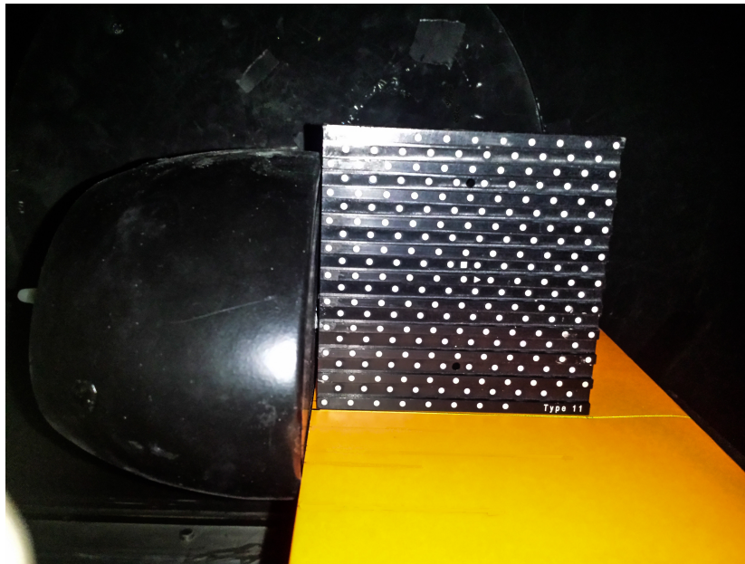
Figure 2.16: Type11 3D Calibration Block used for Stereo PIV and Single Camera PIV measurements
