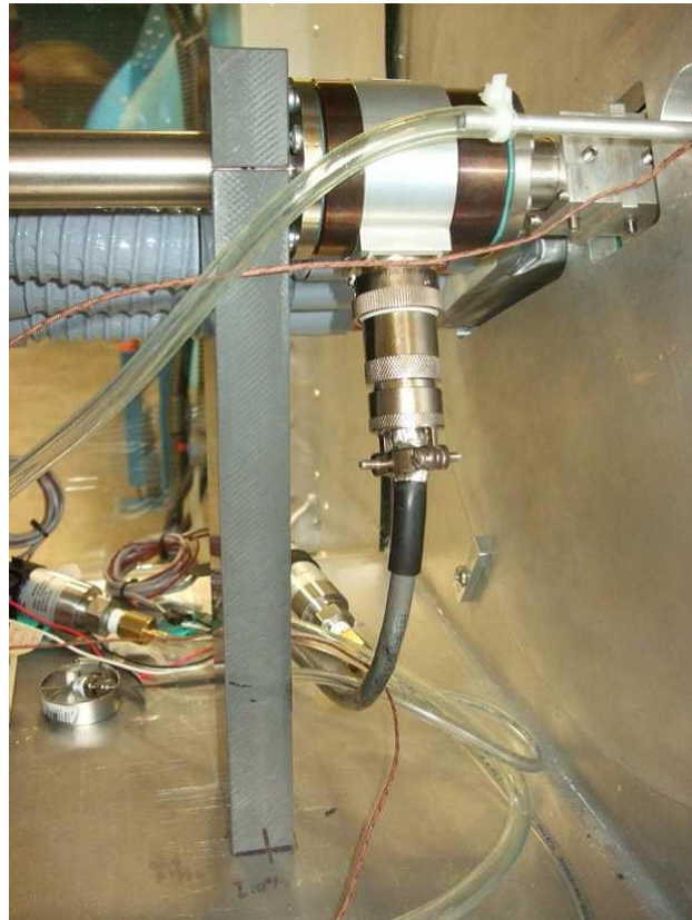
Figure 2.1: Original wind tunnel load cell support column that was redesigned and replaced.
